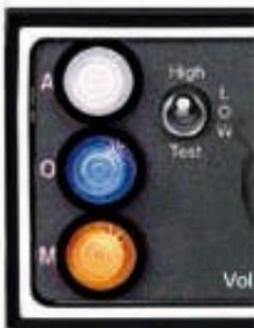
Upon first application of power to the unit, the Marker enters a self test mode. The flickering blue marker light indicates a test in process. If the test continues for more than 10 seconds, or the lamps do not extinguish, return the unit for service.
